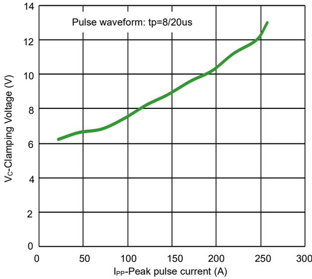
Fig 3. Clamping voltage vs. Peak pulse current
